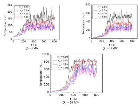
Figure 3. – Temperature curve alone the centerline above the upper room window ( $L_{hp} = 0 \text{ m}$ )
