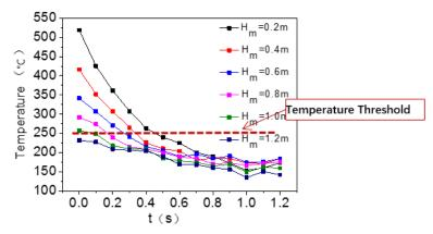
Figure 5. – Temperature distribution of building facade for different fire canopy width and wall height between windows at  $0 < Q^*_{ex} < 1,3$
