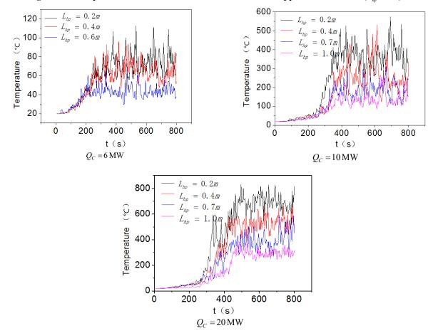
Figure 4. – Temperature curve alone the centerline above the upper room window ( $H_m = 0.4 \,\mathrm{m}$ )
