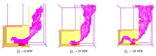
(a) Opening shape B = 0.1 m, H = 0.2 m,  $L_{hp} = 0 \text{ m}$ .  $L_{hp}$  is the length of the fire canopy
