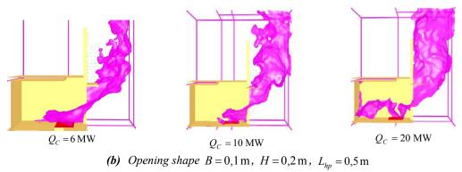
Figure 2. – Isothermal surface at 250 °C
