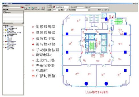
Figure 1. – The operation of the fire control facilities
